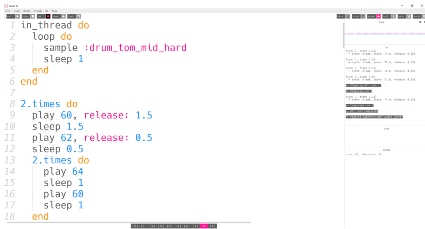
Figure 2: Sonic Pi application interface (version 3.3.1.) with an example of a melodic fragment written with Ruby programming language elements
